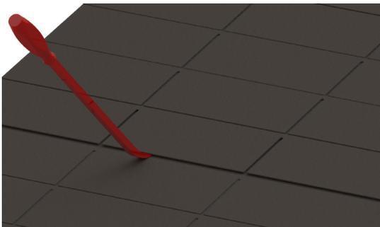
It is important to remove any obstructing nails in the 2nd course of shingles as they can prevent the flashing from extending up under the 3rd course of shingles.
